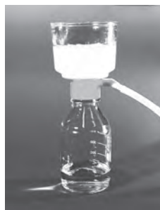
Figure 3: Correct use of the NucleoBond® Bottle Top Filter
